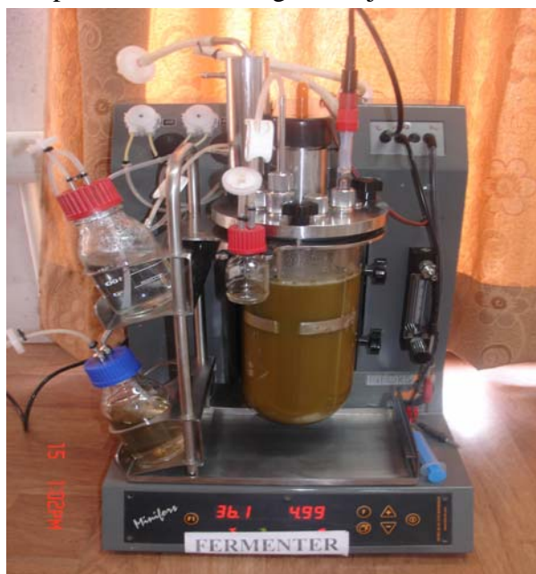
2.5 litre Minifors (Infors HT, Switzerland) fermenter used for ethanol production from sugarcane juice
