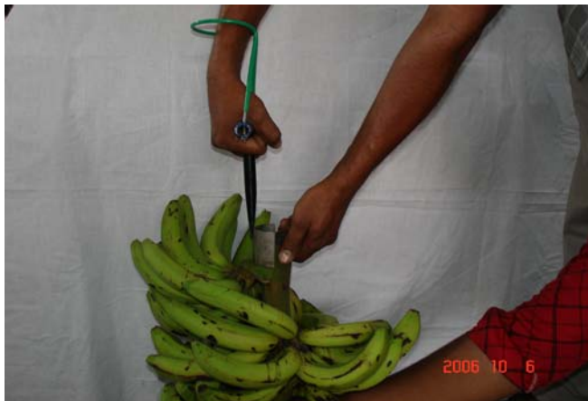
Banana comb cutter in use
