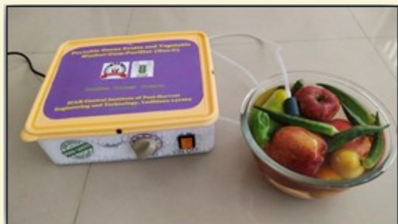
Fig 7: Portable ozone fruits and vegetable washer-cum-purifier (Ozo-C)
