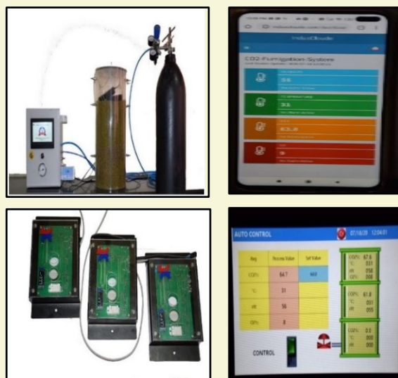
Fig 2: Components of IoT-based smart storage structure for pulses during testing in lab-scale bin
