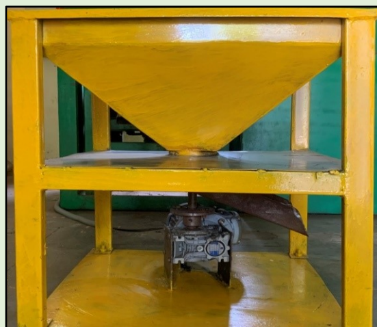
Figure 1 Rotating Orifice Feeding System
