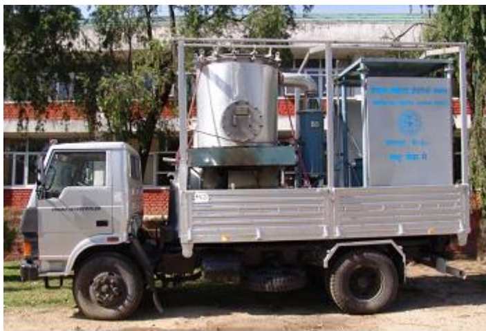
IHBT Mobile Essential Oil Distillation unit
