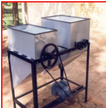
Tamarind Dehuller-cum-Deseeder Machine
