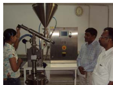
Cryogenic grinder installed at CIPHET
