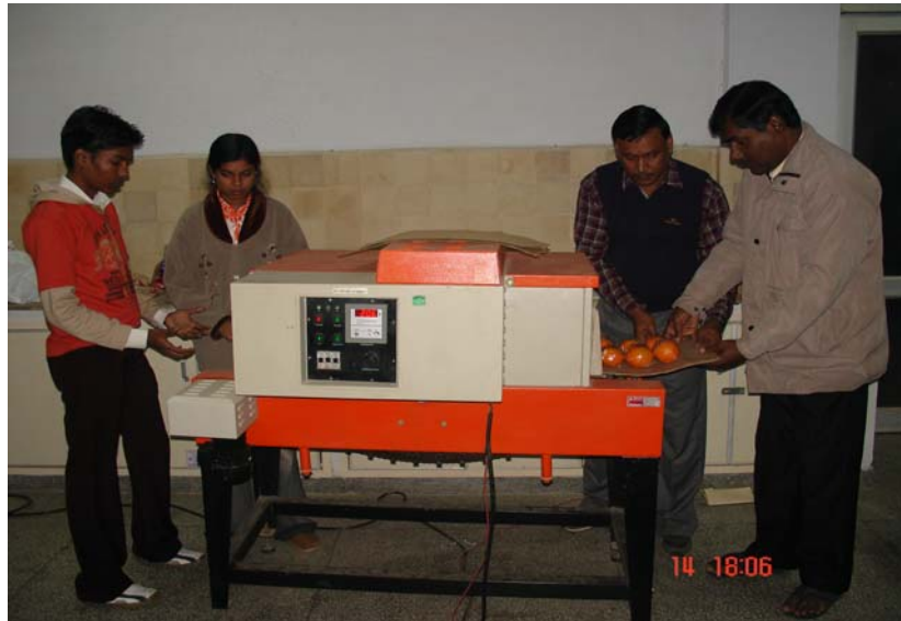
EDP trainees having hands on experience with ISWP (Individual Shrink Wrap Packaging)
