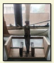
Fig 1. Hand tool mango stone decorticator
