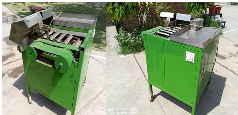
HAU green detopping machine for carrot
