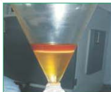
Fig. 67: Phase separation between water soluble and fat soluble fractions of kinnow seed
