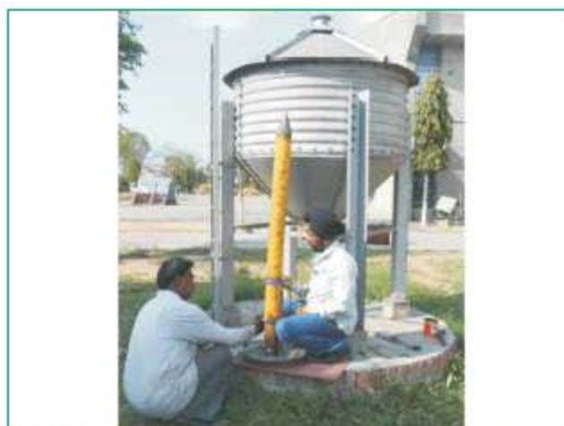
Fig. 28. Multipurpose discharge system for silo
