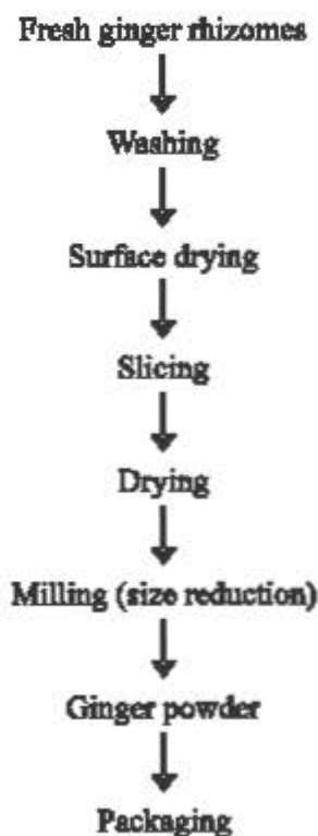
Fig. 84. Process flow chart for ginger processing
