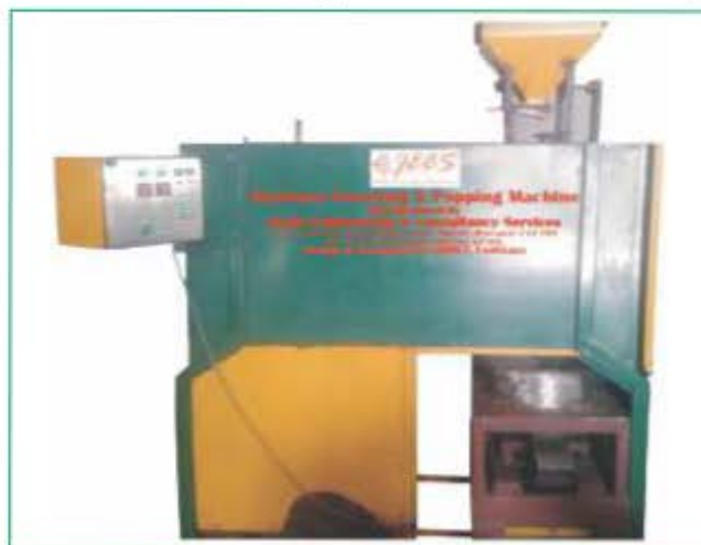
Fig.18. Commercial makhana roasting and popping machine
