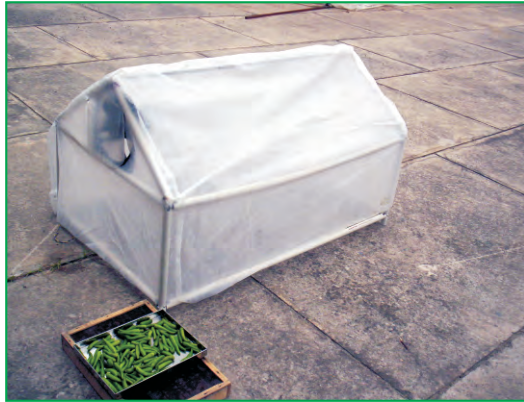
Fig. 58 Experimental setup with drying the chilli in greenhouse
