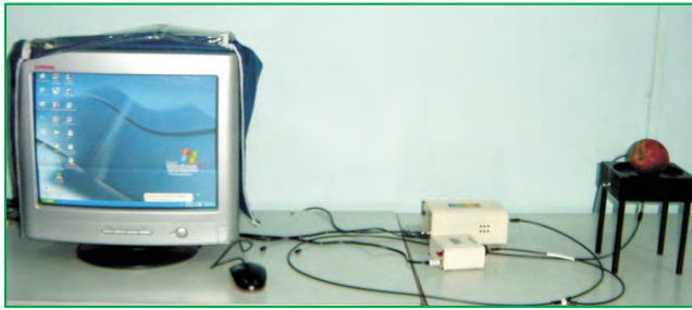
Fig. 1 NIR spectra acquisition setup for apple
