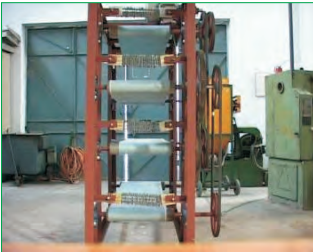
Fig. 74 Side view of the belt dryer
