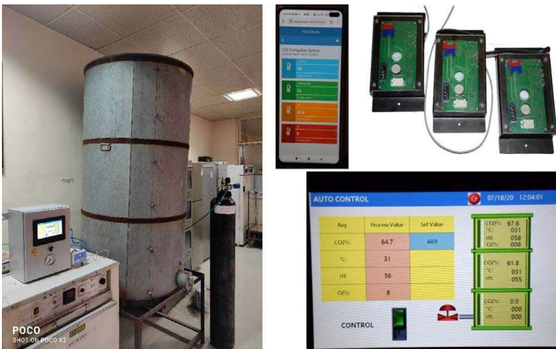
Fig. 5. IoT-based Smart Storage Structure for Pulses with Sensor module, HMI display for monitoring fumigation parameters from cloud and control panel
