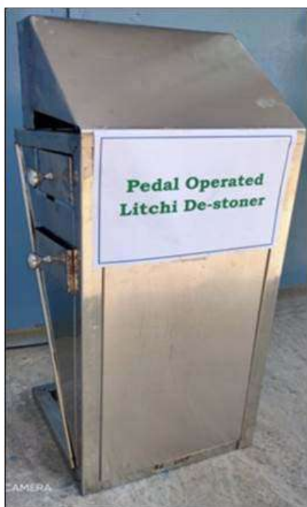
Fig. 8. Pedal operated litchi seed removing tool
