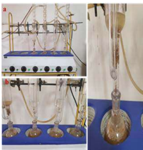
Fig. 31. Conventional extraction using different solvents a) Ker powder; b) Sangri powder
