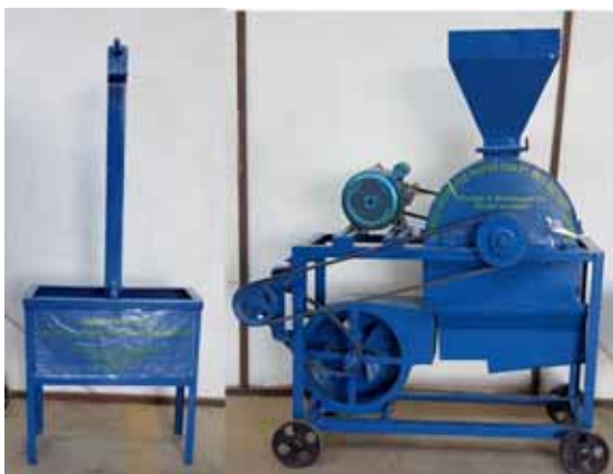
Hand and power operated Water chestnut decorticator
