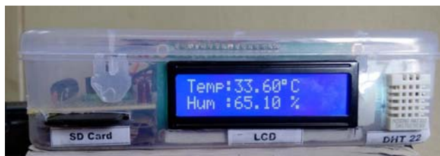
Fig. 4. Overall setup of the designed data-logger
