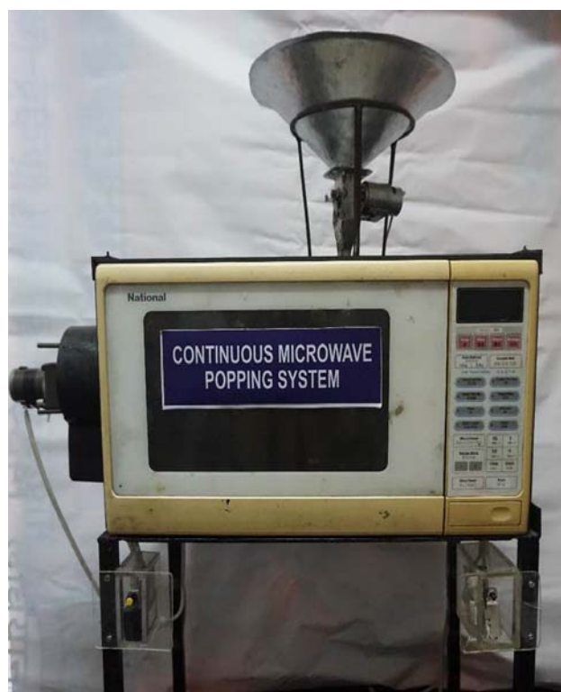
Fig. 7. Continuous microwave popping system
