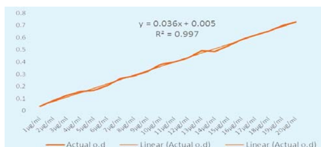
Fig. 35. Standard curve for detection of metanil yellow Y = mx+c , where x is concentration of metanil yellow in (µg/ml) and Y is absorbance at the given maxima
