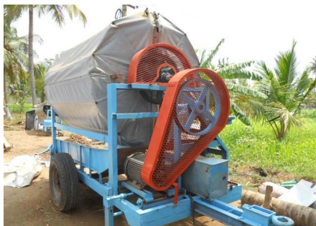
Fig. 46. Turmeric dust free polisher
