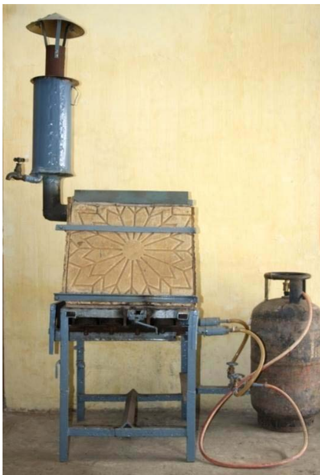
Fig. 47. Chunga chawal making machine
