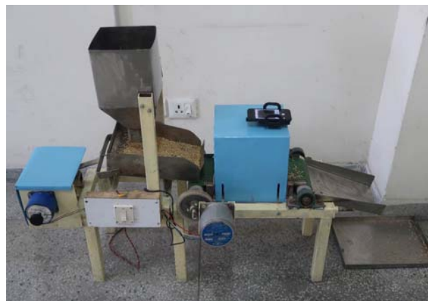
Fig. 5. Isometric view of device for automatic detection and identification of insect infestation and level of infestation
