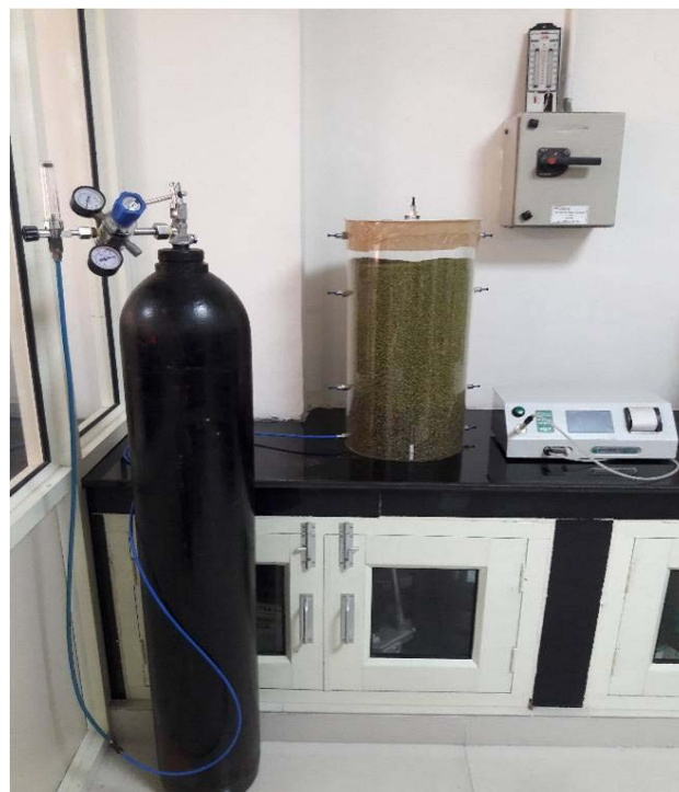
Fig. 12. Hermetically sealed storage structure
