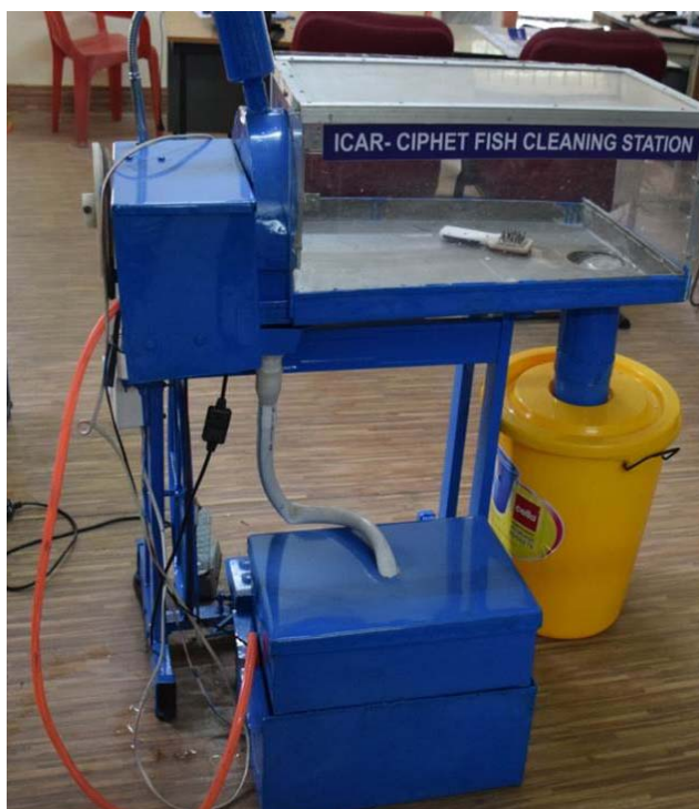
Fig. 10b. Final Prototype of Fish Cleaning Station
