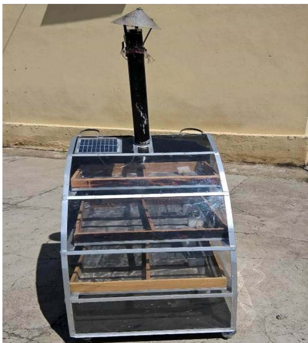
Fig. 52. Solar cabinet dryer
