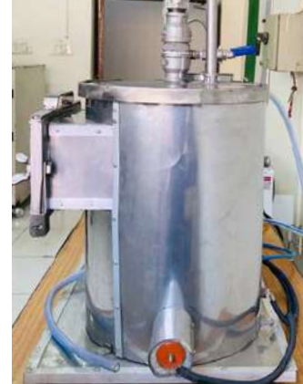
Fig. 1. Table-top Vacuum Frying System
