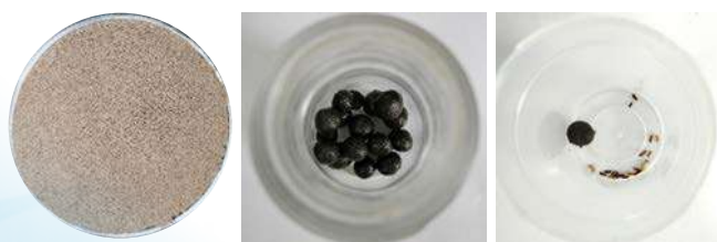
Fig. 11. Mustard based Substrate for Tablet, Formulated Tablets and the Mortality of Exposed Insects
