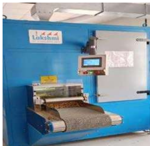
Fig. 42. RF System for Treating Turmeric Rhizomes
