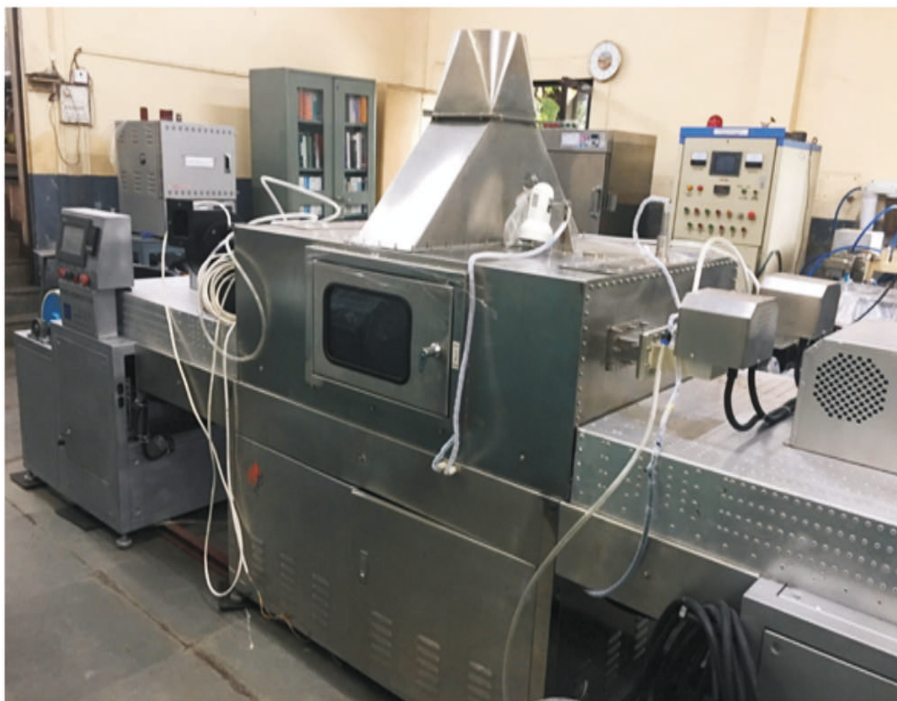
Fig.26. Continuous microwave disinfestation system for rice & wheat
