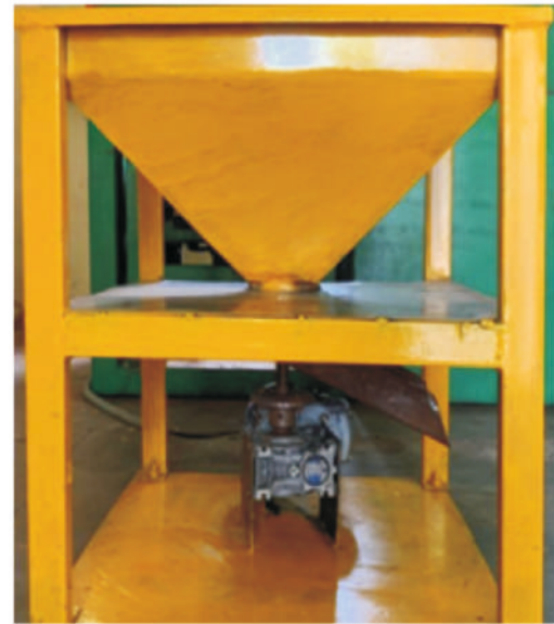
Fig.3. Feeding system for Continuous and uniform discharge of makhana seeds
