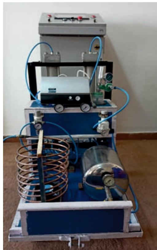
Fig.4. Oxygen concentrator for ozone generation
