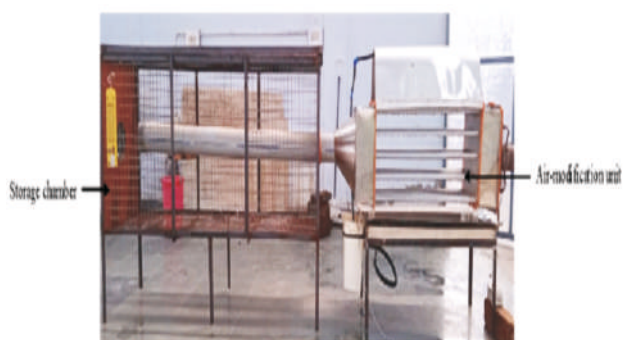
Fig.6. Onion storage structure
