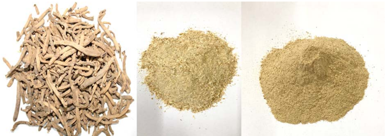
Fig. 15a. Cryogenically and ambiently ground powder of safed musli roots (a: cryogenic b: ambient)
