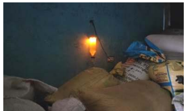
Fig. 25 b. Light trap prototype installed in a flour mill at Hambran Road, Ludhiana
