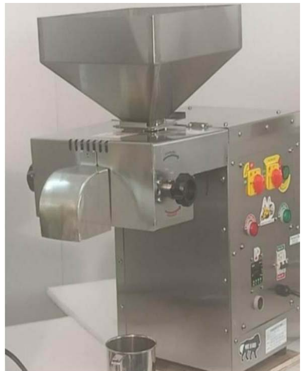
Fig. 31. Cocoa butter extractor schematic diagram and developed machine
