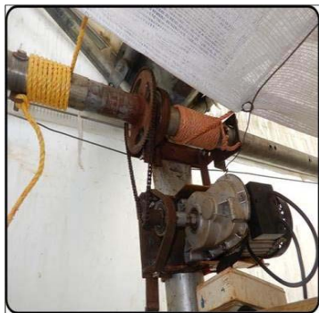
Fig. 45a. Clamps and nut bolt fitting system to the chain sprocket and motor fitting of the automatic shading system
