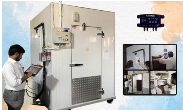
Fig. 30. Micro-climate storage bin for groundnut pods
