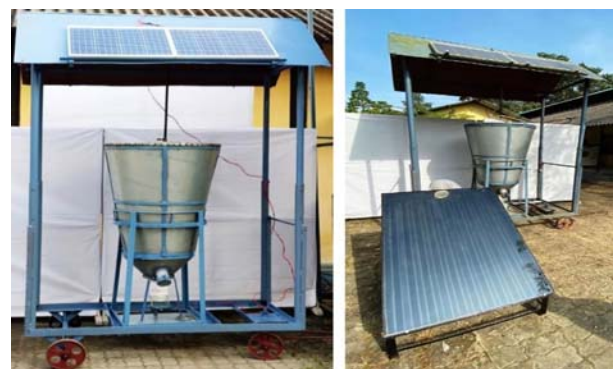
Fig. 29. Storage bin with an insect trapping device and solar heating system
