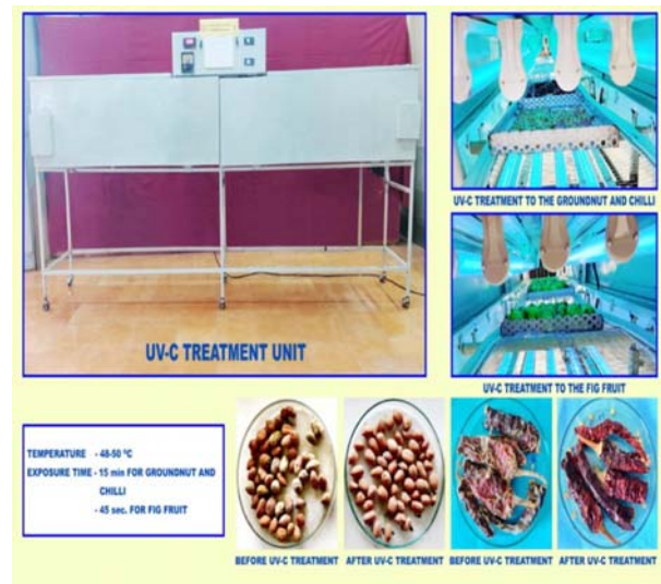
Fig. 32. Continuous type UV-C treatment unit with samples
