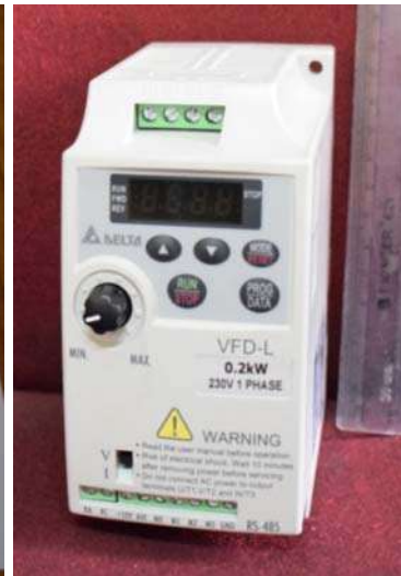
Variable frequency drive (VFD)
