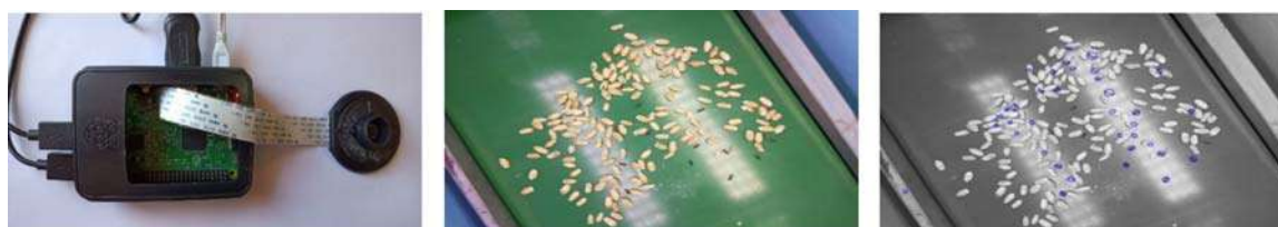
Fig. 53. Smart device for detection of insect pest in stored grains (a. Raspberry Pi board with camera V2, b. Captured image of infested grain and c. Image with detected insects/blobs)
