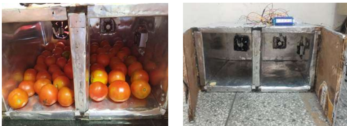
Fig. 56. Multi-cold storage chamber using peltier module
