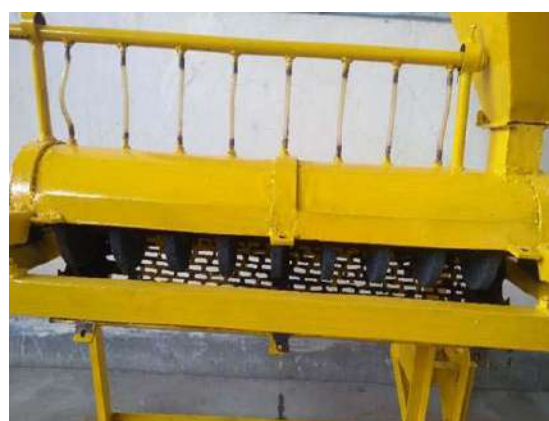
Fig. I. Continuous makhana seed washer
