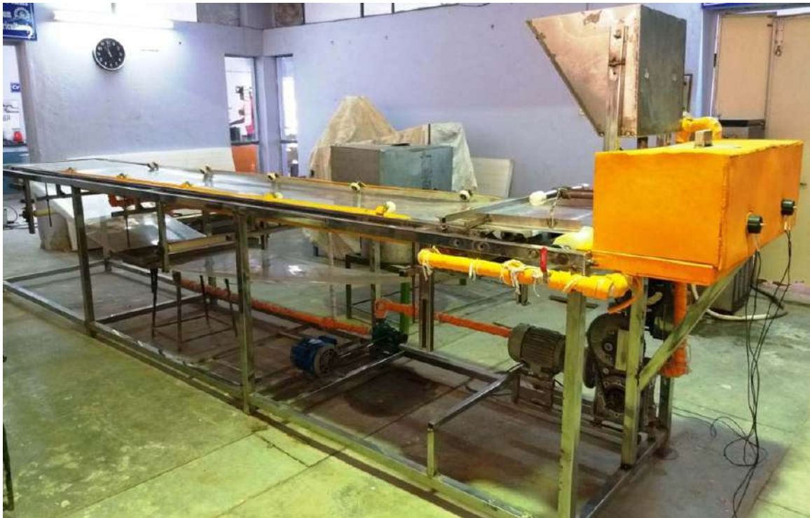
Fig. 2. Pictorial view of assembled refractance window dryer
