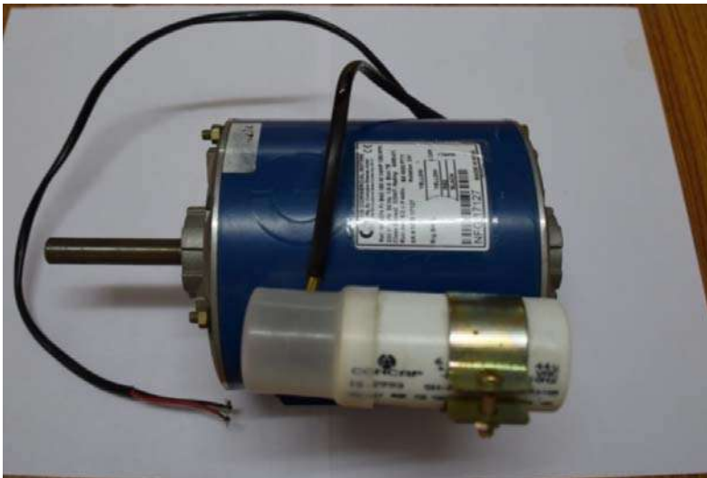
Single phase AC motor ( \frac{1}{4} HP, 1380 rpm)
