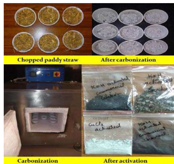
Fig. 24. Fig. showing carbonization and activation of charcoal
