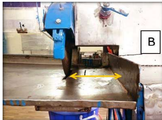
Cutting clearance after modification (B)
