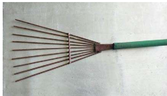
Fig. 2. Hand tool for stirring makhana seeds during initial roasting
