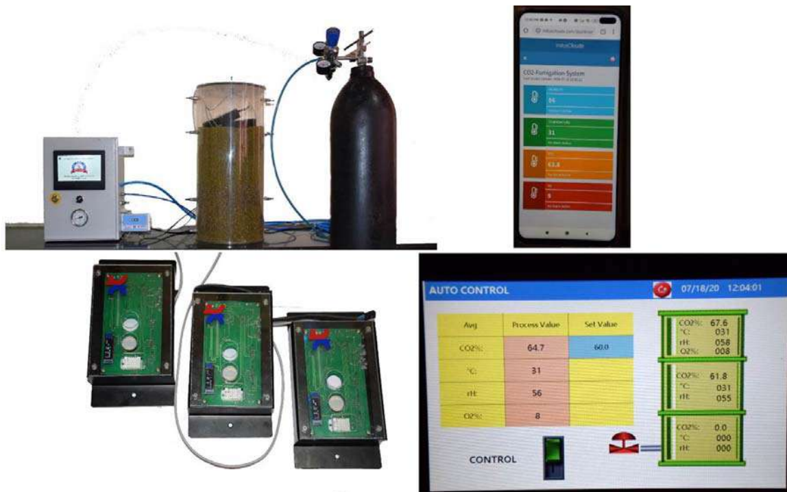
Fig. 27. Components of IoT-based Smart Storage Structure for Pulses during testing in lab-scale bin
