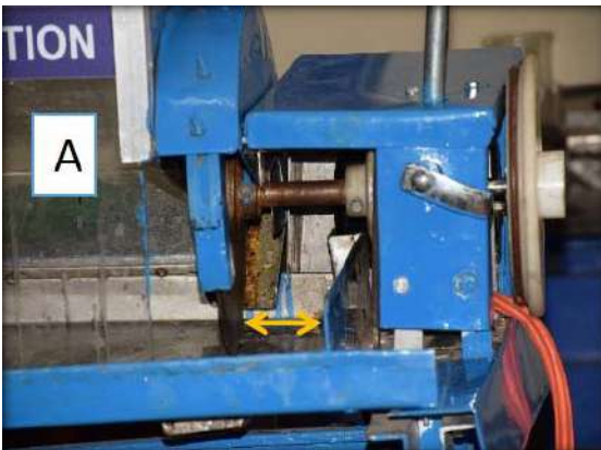
Cutting clearance before modification (A)
