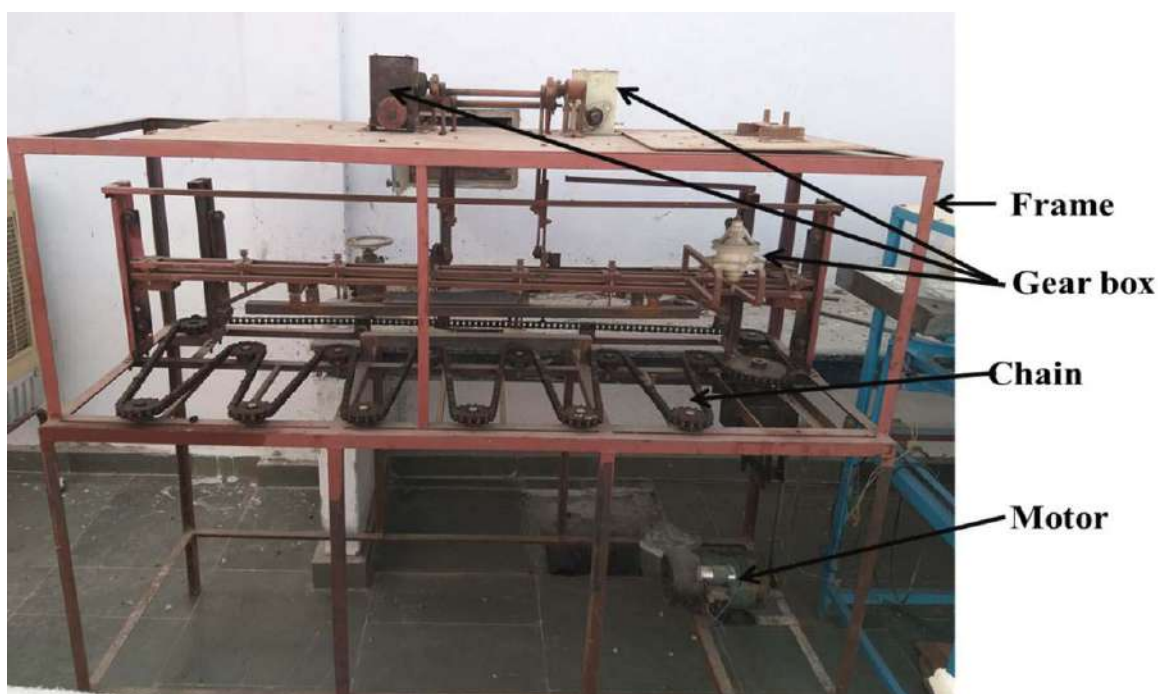
Fig. 10. Pictorial view of the framework with components of the prototype
