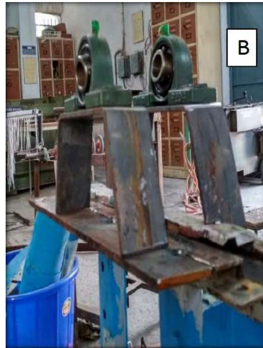
Bridge for mounting the bearings before modification (A), after modification (B)
