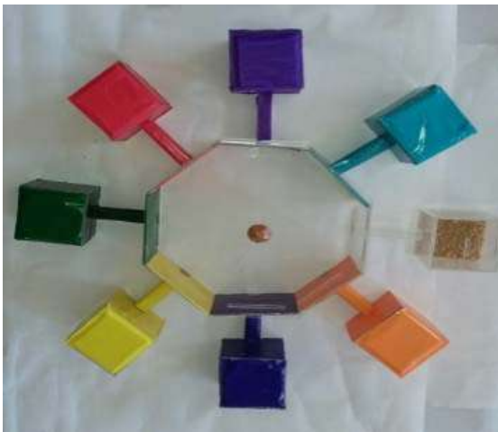
Fig. 1. Acrylic insect experimental set for colour cue preference test
