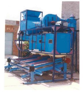
any further manual grading. The medium and light fractions can be used for oil extraction. The machine runs on 3 kW electric motor, requires two people to operate. The cost of the machine is approx. Rs. 2,00000/- and capacity is 650 kg/h.
